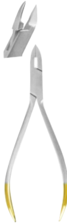
Soft Wire Cutter & Ligature Cutter, Micro with TC tips. Cuts Wire 0.23 mm to 0.30mm 04-2065
