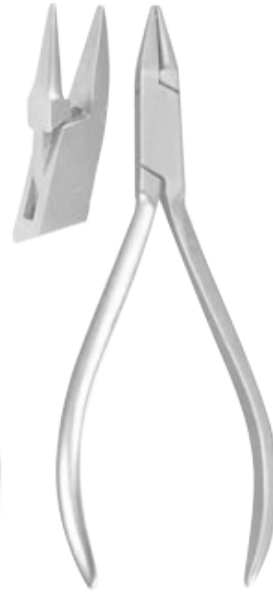
Adams Plier mixi used for prices right angle bends and appliance adaptation up to 0.040" 04-2034
