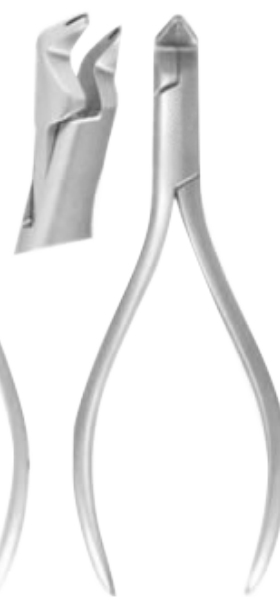
Crimping Plier angled used to crimp surgical ball hooks to archwire, slotted tip fits cover base of hook for secure hold while crimping 04-2030
